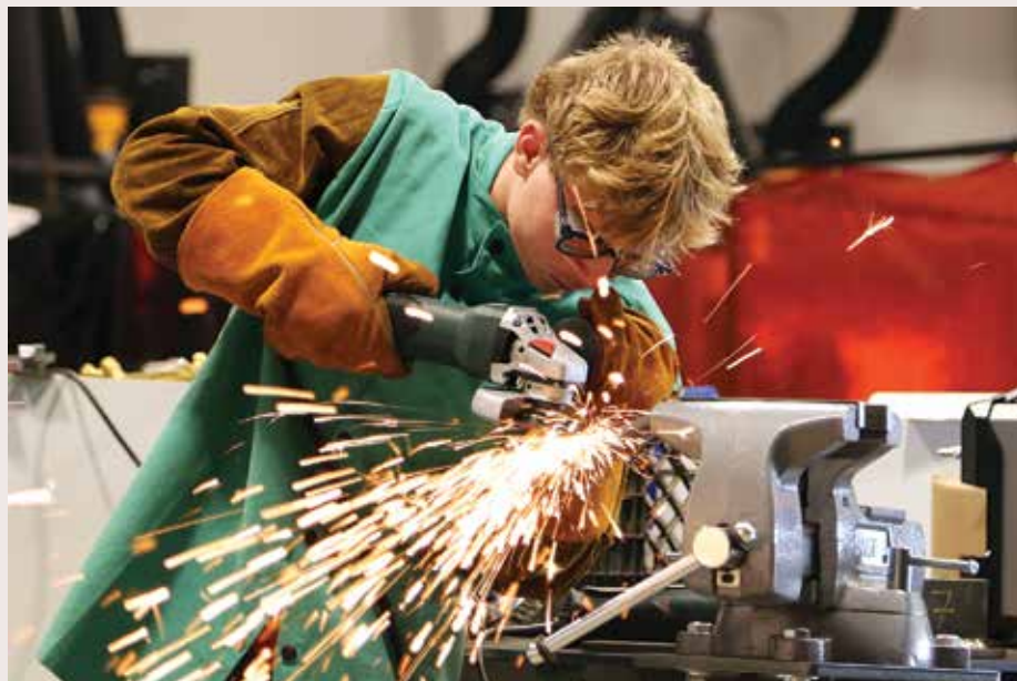
Above: Donny Daugherty, a junior at Lincolnwood High School in Raymond, Ill., uses an angle grinder to prepare metal for welding in Matt Belusko's metal fabrication class.
